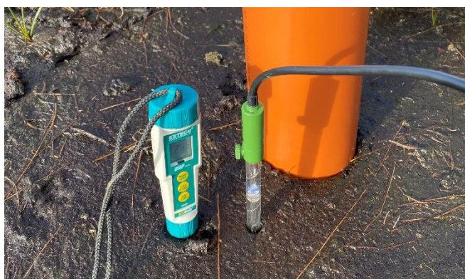
Figure 4: Accessible pH and Eh probing methods.
